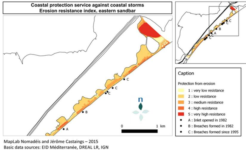
Figure 22: Map of the erosion resistance index for the eastern Etang de Pierre-Blanche sandbar
