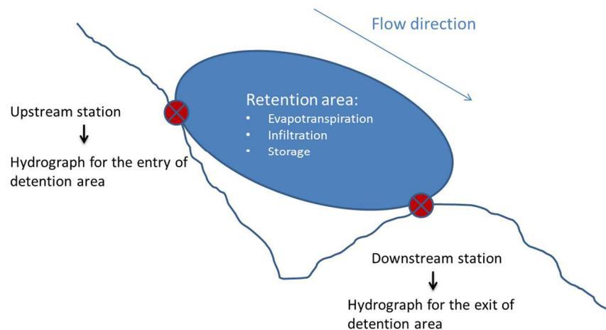
Figure 34: Diagram showing the hydrograph method: comparison of retention area input and output hydrographs
