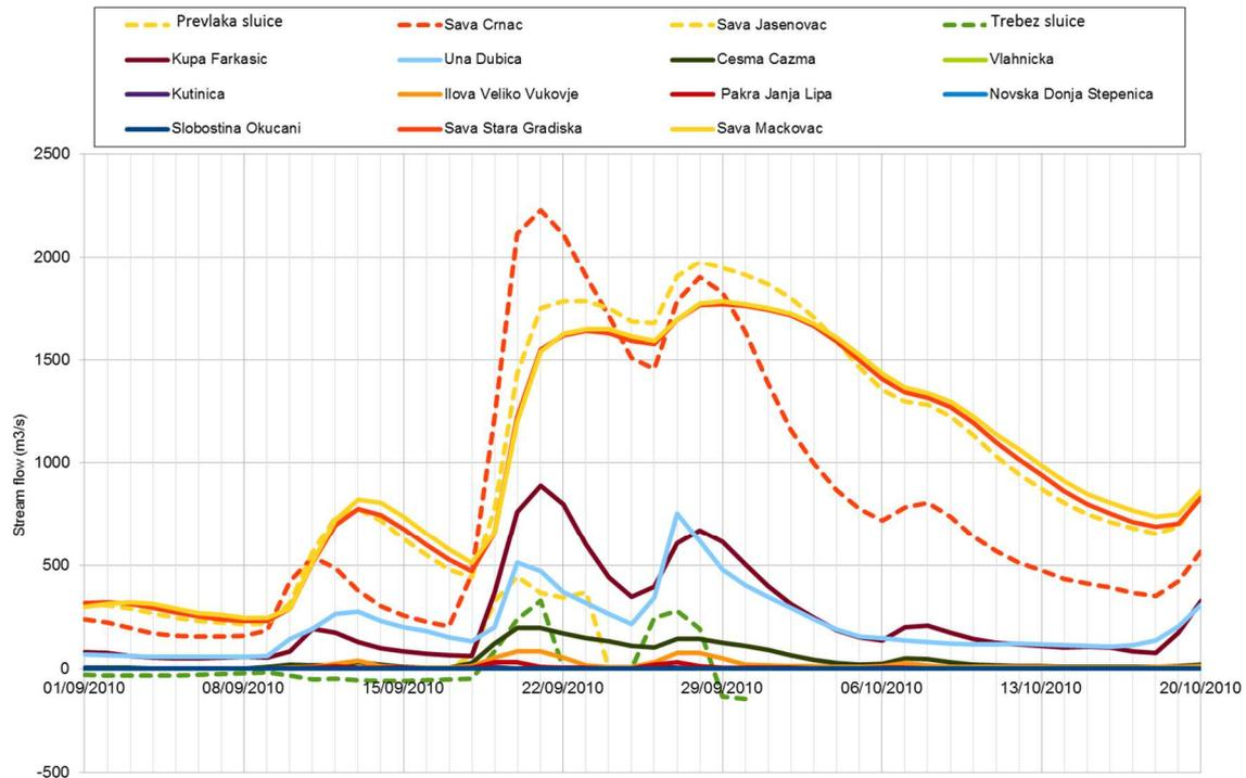
Figure 35: Daily variation in flow rate recorded by 15 measurement stations during the September 2010 flood
