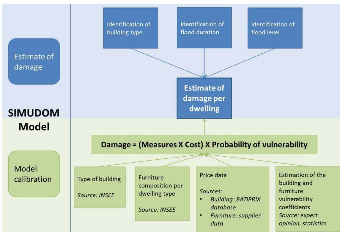
Figure 31: Functional diagram of the SIMUDOM model (Nomadéis illustration based on CEPRI, 2014)
