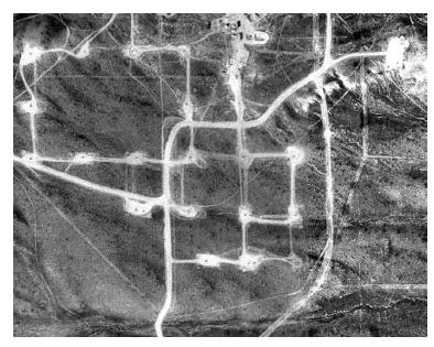
FIGURE 10.1 Roads built for oil and gas development in the sagebrush landscape of the western United States show up clearly in this digital air photo (Weller et al. 2002).
