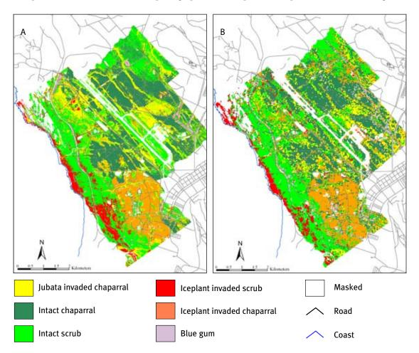
FIGURE 11.7 Classification of six vegetation types at Vandenberg Air Force Base, California, USA: A. Hyperspectral (AVIRIS) image (4 m and 174 wavebands) and B. Landsat ETM (30 m and 6 wavebands)<sup>3</sup>.
