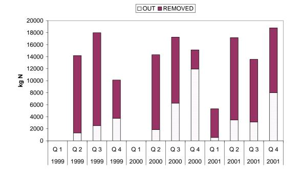
**Figure 3.** Quarterly load, removal and outflow of tot-N at wetland Alhagen, Nynäshamn, receiving chemically treated municipal wastewater. Total area of the wetland system is 28 ha. The data for quarter 1 in 2001 are from March only.
