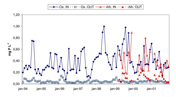
**Figure 1.** Inflow and outflow concentrations of tot-P in the FWS wetlands in Oxelösund and Alhagen, Nynäshamn, receiving chemically treated municipal wastewater.
