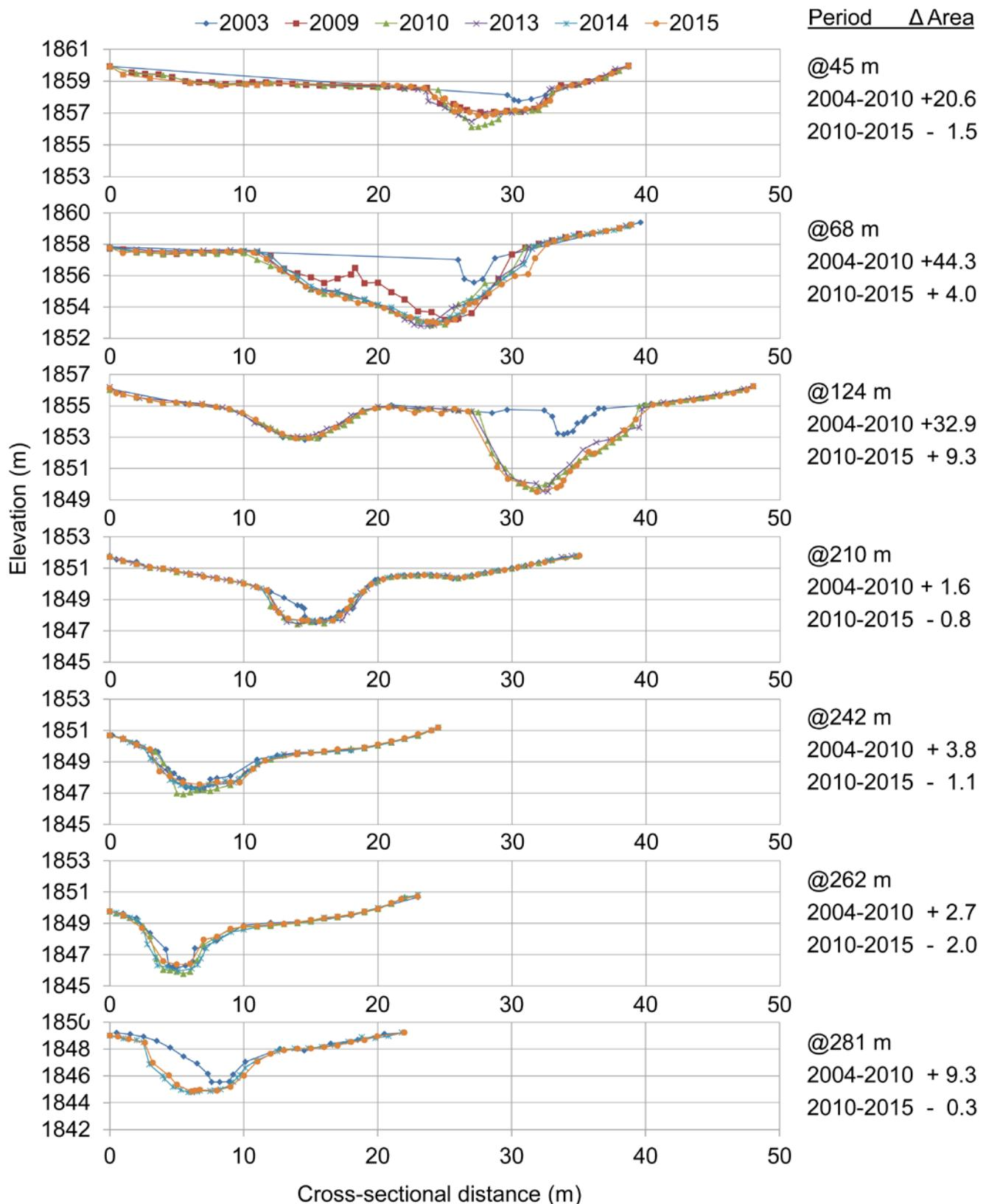
Figure 6. Repeated cross-sections at Turkey Spring site, downstream view, with changes in cross-sectional area ( $m^2$ ) between sampling periods (positive values signifying erosion, negative values signifying filling).
