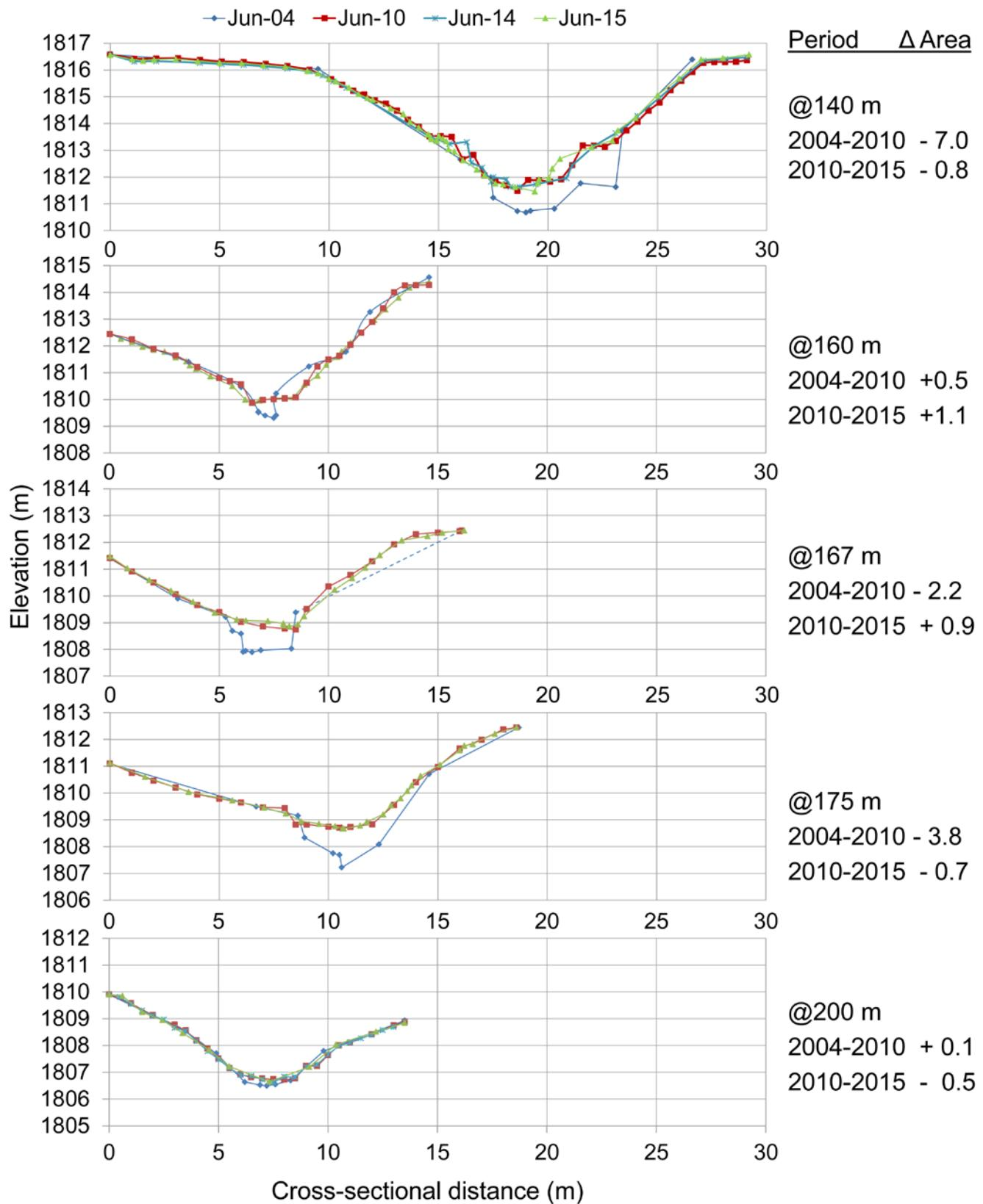
Figure 7. Repeated cross-sections at Swamp Spring site, downstream view, with changes in cross-sectional area ( $m^2$ ) between sampling periods (positive values signifying erosion, negative values signifying filling).
