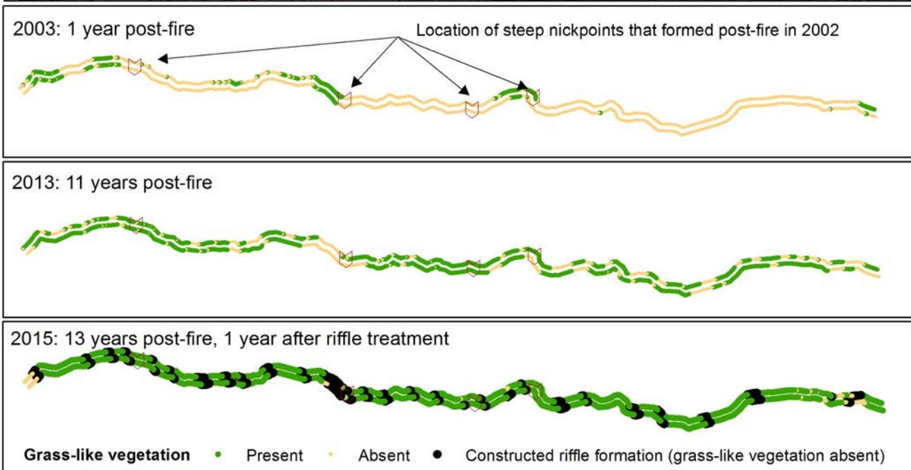
**Figure 3.** Planform view of the Turkey Spring site overlaid on an aerial photograph (post-fire, 2012) showing the reference points for monitoring, including locations of cross-sections, steep nickpoints and photopoints. Surveys along the 550 m reach recorded changes in the presence of grass-like vegetation and the location of riffle formations that were placed in 2014.
