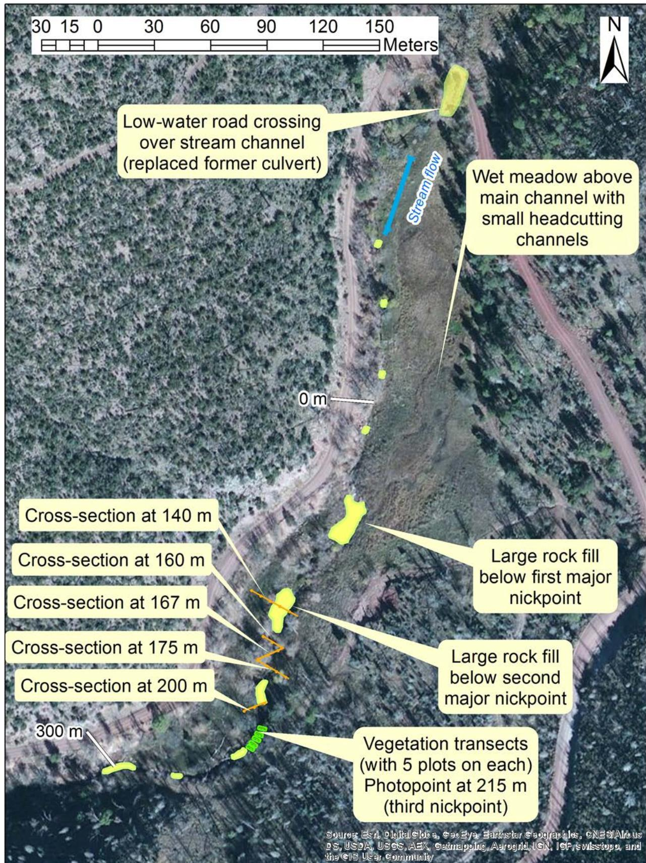
**Figure 4.** Map of the Swamp Spring site (Arizona, U.S.) showing the reference points for monitoring, including locations of cross-sections, riffle formations, vegetation plots, and a photopoint, overlaid on an aerial photograph (post-fire, 2012).
